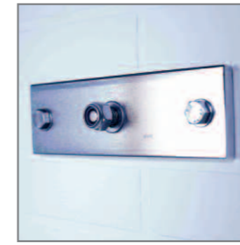
UP0112A Wall Anchor Plate – 316 stainless steel, electro-polished. 50kN min breaking strength
