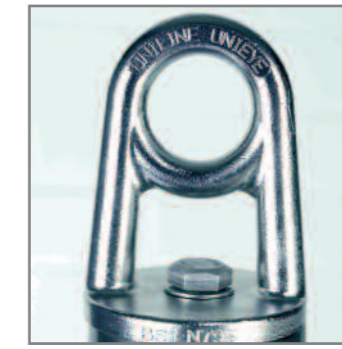
UE0100A Unieye end anchorage connector – 316 stainless steel, electro-polished, serial numbered – 67kN min breaking strength
